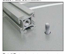
Detail D: Attach vertical extrusions to base plates using supplied bolts inserted through the hole in the plate. Be careful not to strip the thread.
