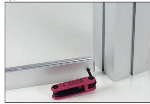
Detail A: Most horizontal extrusion connections have a patented expandable lock. This lock inserts into the groove of an opposing extrusion. Tightening the lock with the hex key tool expands the lock and creates a strong connection.
