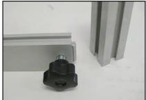
Detail F: Plastic knobs are used to tighten locks where horizontal extrusions connect with vertical extrusions. Turn the knobs clockwise to tighten. Turn counter-clockwise to loosen, but do not remove knob.
